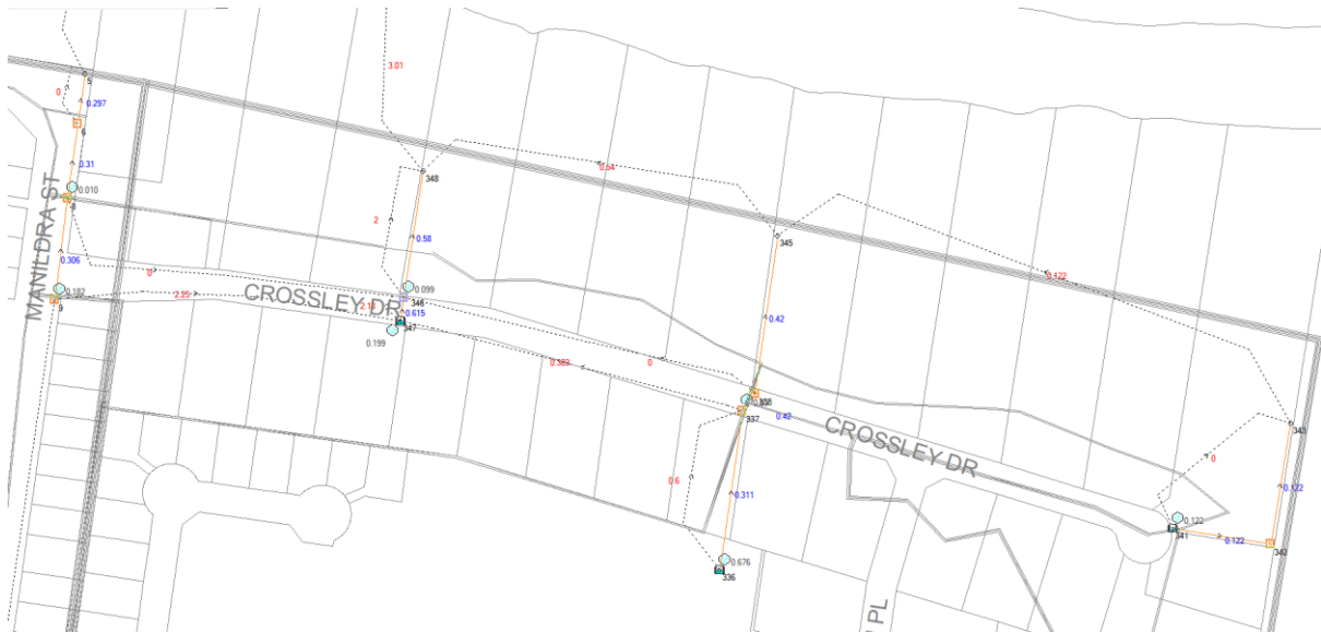
Figure 16 Existing DRAINS 5yr ARI Results (Catchment C8) – Drainage at 7, 13 and 29 Crossley Drive Peak catchment flow rates in m 3 /s are given black , pipe flows in blue and overflows in red
